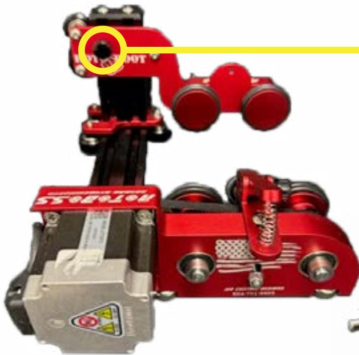
Loosen this thumbscrew, and manually move arm up/down to your desired position for engraving items.
