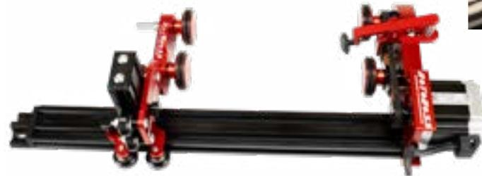
Loosen this thumbscrew, and manually move arm side to side to your desired position to align items on all wheels for engraving.
